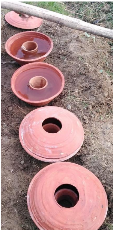
Plate 3: Testing the cocoons for cracks and defects through the water leakage test.
